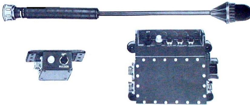
*Above is the stalk, with the detectors mounted within the dome at the right, the thickened section is of rubber which allowed some flexibility. Below, the larger unit is the main control unit, and the smaller unit housed the buzzer and warning light.*
