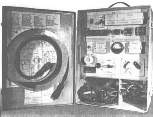
The amplifier in its case. The cable on the left supplied the optical unit. On the right, is the amplifier, power unit (110/220 AC or 12 DC), and switching to allow connection to an external telephone circuit.
