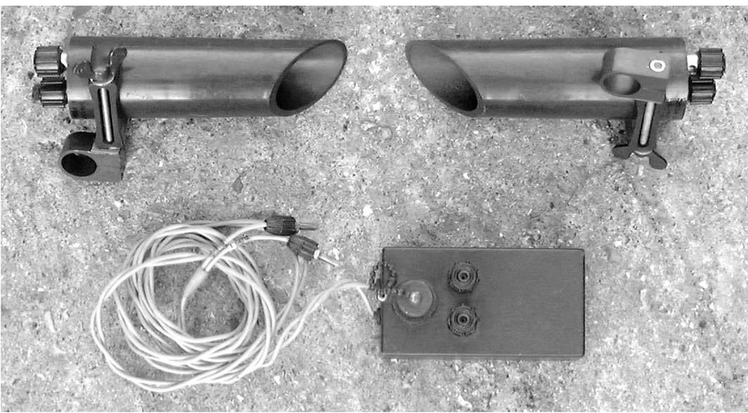
*On the left is the IRIS transmitter, which externally appears very similar to the sensor on the right. To try to avoid confusion each was embossed with 'T' or 'S' in unnecessarily small type. The alignment aid is below, with a pair of wires, which were plugged into the sensor. Once aligned the unit was unplugged, and the sensor was connected via D 10 wire to the main control unit.*
