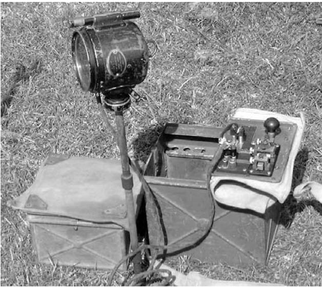
*Lamp Signalling Daylight Short Range Projector Mk II with its carrying case which stored the battery. When opened the lid provided a solid base for the Morse key. The box on the left contained spares and filters.*
