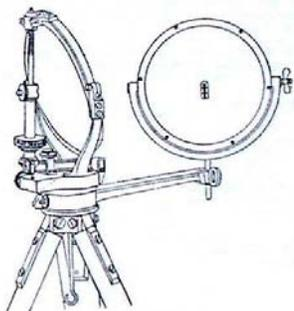
*Where the sunlight is shining from behind the sender a second 'duplex' mirror is needed to realign the beam.*
