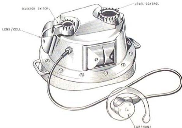
*Controls on the infra-red detector*
