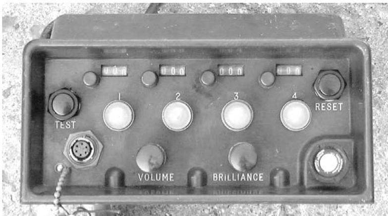
*The monitor unit, at the top can be seen the hinged cover to protect the terminals that connect to the sensors*
