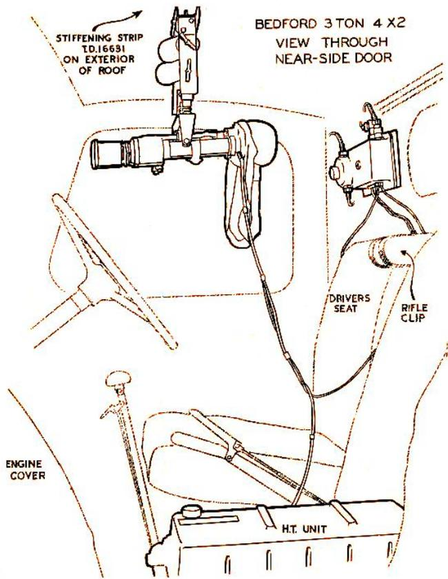
Generally in trucks, the binocular supporting frame was secured to the cab roof.
