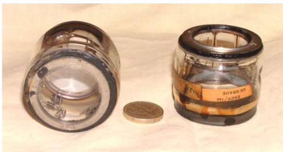
*Two converter tubes type CV144 either side of £1 coin. The converter tube on the left shows the viewing screen (the cathode) at the far end of the tube, the fixing of the screen to the tube is particularly delicate, although the outer glass tube is more resilient. The other vulnerable part is the cathode connection from the tube to the HT supply; it consists of a paper ring painted with graphite. Removing the tube, particularly after many years, can easily pull the paper away.*
