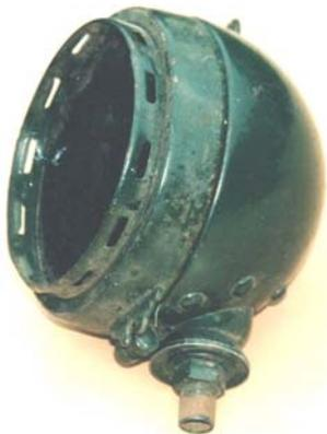
*This shows a Tabby headlight, the infra red filter can be seen obscuring the reflector, the clear plastic diffuser is not fitted here.*
