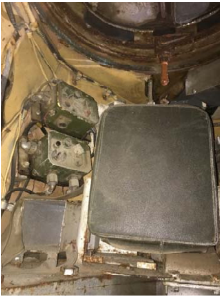
Figure 5. The interconnecting box, radio-line (top) and the 'I' box (bottom) next to the No. 1's seat in the turret
