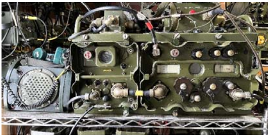
Figure 17. The C45 A-set, mounted on to a standard Larkspur tray/carrier type 82, and also showing the ALS26 loudspeaker unit gun control at the left hand side – together with its Handset SI No. 7B
