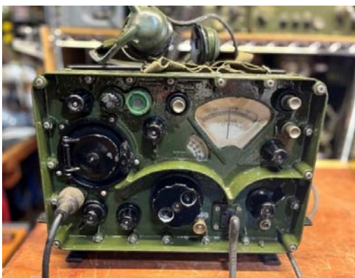
Figure 19. The R209 Mk 2 reception set used for reception of meteorological data
