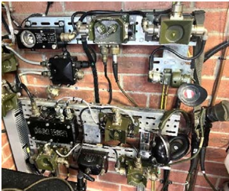
Figure 26. The driver's 'D' box can be seen at the top centre, with his Microphone Magnetic SI No. 6 and Amplivox E22 noise-reducing headphones hanging on the right. Also visible is a '6T' box and two 'LT' boxes, and the ECC emergency crew control box top left - the (external) induction loop associated loudspeaker is just out of sight above the ECC unit
