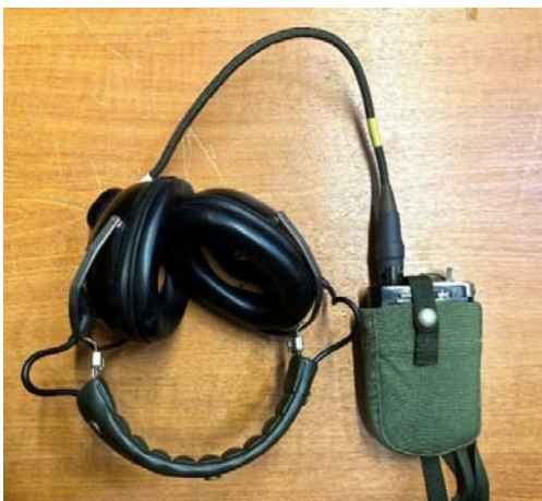
Figure 31. A pocket induction receiver – Receiver, Induction No. 1 - together with the Amplivox noise-reducing headphones
