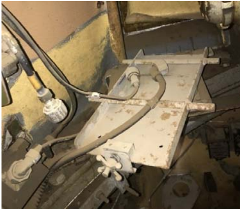
Figure 4. The radio tray, with the radio ( Clansman ) long since removed, as well as other radio items that were on the inside of the turret wall. Note the original installation with the B48 would have used a carrier type 81 for mounting
