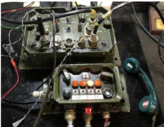
Figure 11. The author's 'home-made' Abbot test box, with the gun control unit and the CPO's handset undergoing test
