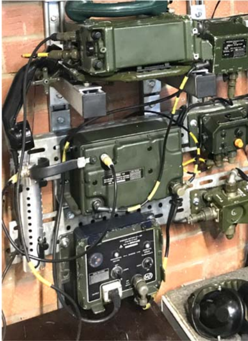
Figure 23. The UK/PRC-351. Note the additional Clansman items – the 24 V battery (fitted to the radio set), DCCU battery charger, TUAAM automatic antenna matching unit and initiate box: the Interconnecting Box Radio Adapter - IBRA box (top right) interfaces the Clansman radio into the existing (original) Larkspur harness, the output of the IBRA feeding directly into the Larkspur radio-line box. To the left of the Clansman's TUAAM unit is the 50 \Omega dummy load
