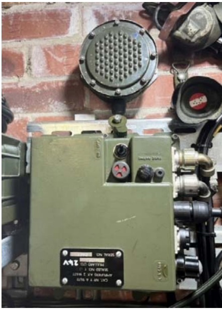
Figure 13. The 2 W amplifier and the 3 Ω 5” loudspeaker
