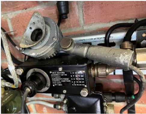
Figure 28. The ECC box with the Tannoy microphone plugged in. Note the microphone will be stowed when not in use
