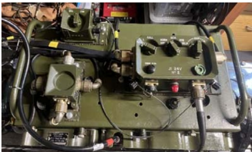
Figure 18. The top of the C45 A-set showing the 'MRRB' box (top left) and 'J1' box – items 18 and 17 respectively. The box at the bottom left is one of many 'LT' 24-volt distribution boxes, none shown in Figure 9 for clarity. Note the items are assembled onto a standard Larkspur top tray for this type of set
