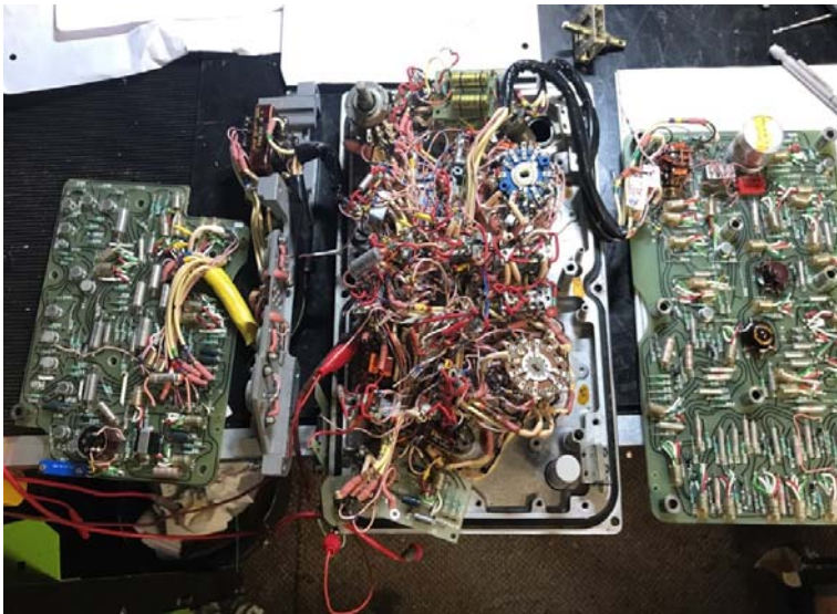
Figure 9. The DM box opened out together with the power transistor and transformer assembly hinged open, and the main chassis area in a state of 'disassembly'
