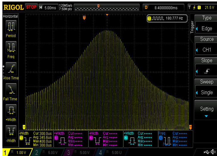
Figure 20. The bandpass filter, centred on 1.9 kHz (passband \pm 600 Hz) as used on the TEST DM function
