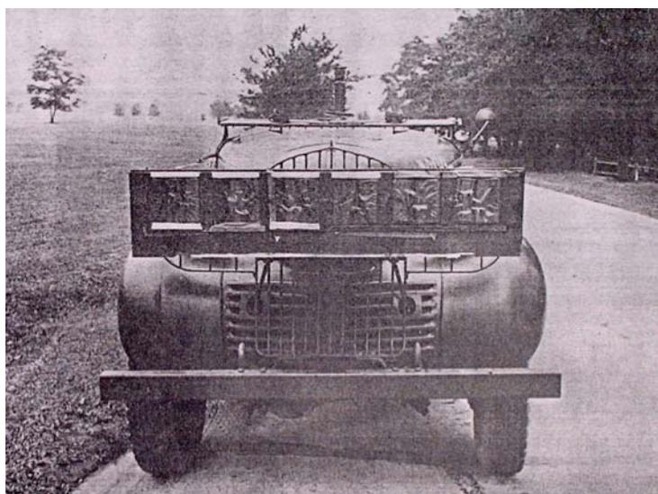
*An early system of IR headlights fitted to a Dodge VC-5 pickup in August 1940.*
