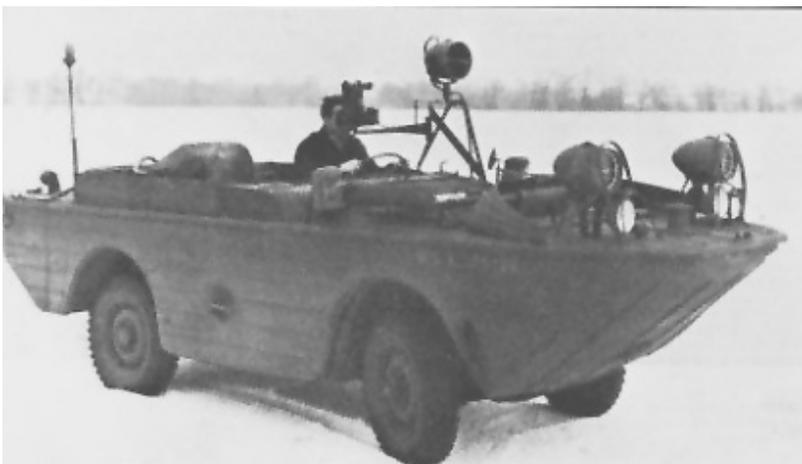
*Ford GPA with periscope type viewer. Note IR spotlight & IR headlamps requiring 1.5kW onboard generator.*
