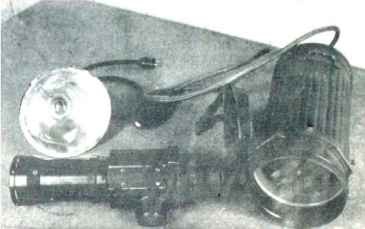
*To the left is the bildwandler rifle sight, above that the lamp and reflector which has been dismantled from the lamp box and filter on the right.*
