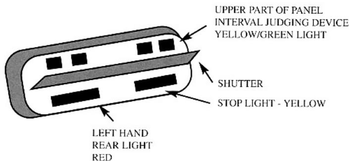
*Rear interval-judging panel and stop light fitted on left-hand rear of vehicle*
