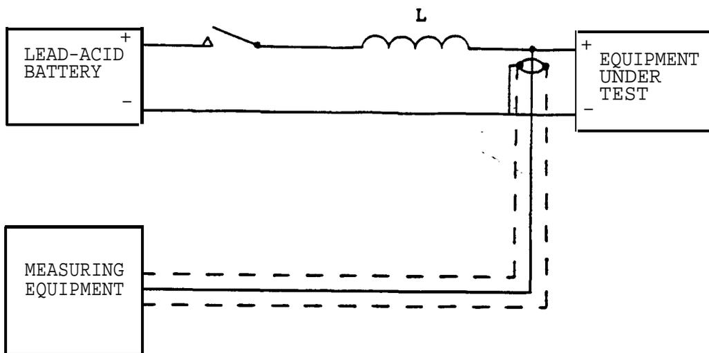
NOTE: L =  $5\mu\text{H}$  for the simulated 'Generator Plus Battery' Condition or  $50\mu\text{H}$  for the simulated 'Generator Only' Condition.
