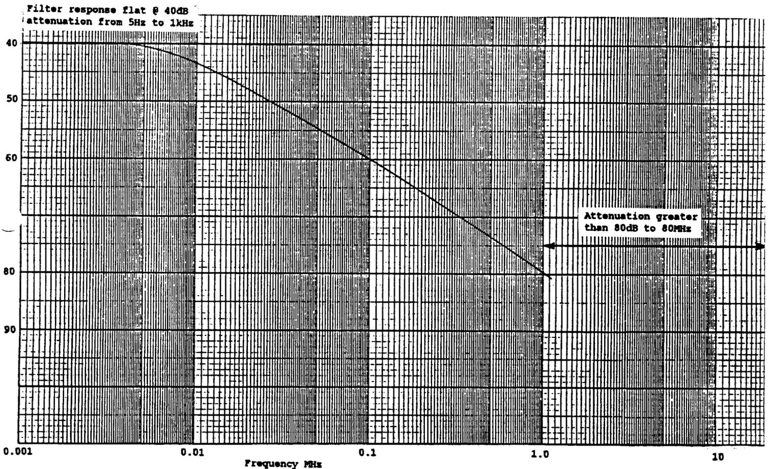
Fig B.1b Typical Frequency Response of 10kHz Filter + 3m Cable
