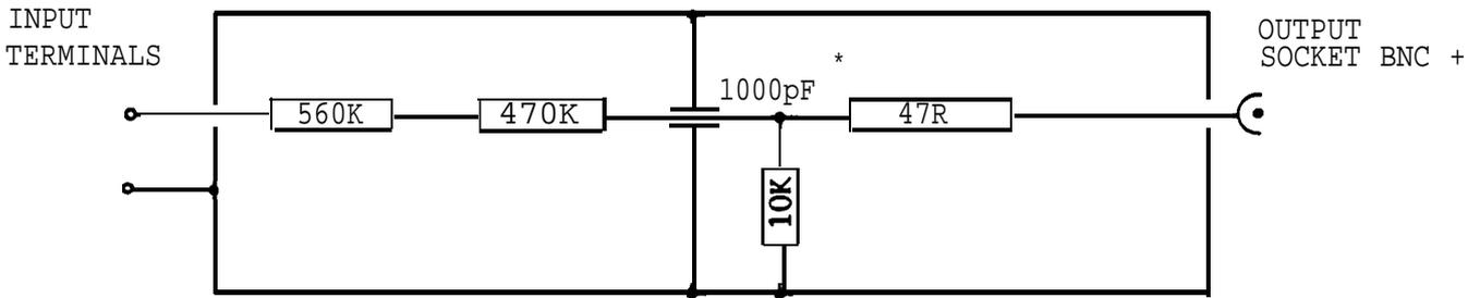
\* 1000pF lead thro' capacitor value adjusted on test to give 3dB bandwidth of 10kHz  $\pm$  10%.
